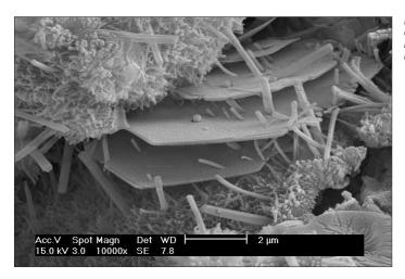
Hydration of a Portland cement-based binder in a traditional grouting mortar
